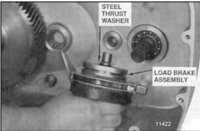
Figure 5-5. Removed Load Brake Assembly.
